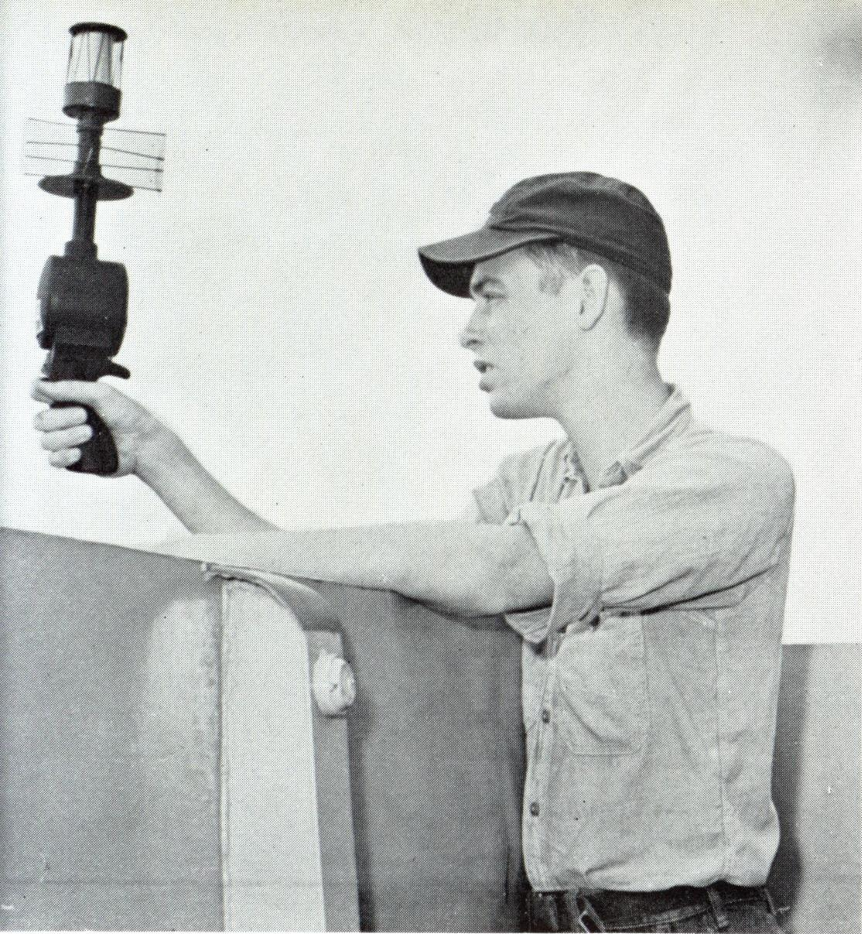
It looks like an atomic-ray gun, but is used to measure wind velocity.
